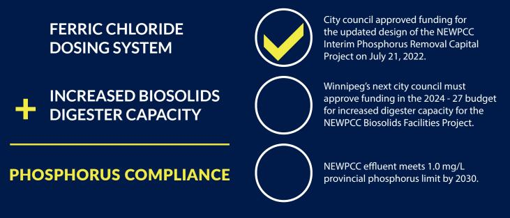
**HOW PHOSPHORUS REMOVAL WORKS:** Ferric chloride binds to phosphorus and settles out of the liquid waste. The resulting solid waste is treated by increasing biosolids digester capacity.
